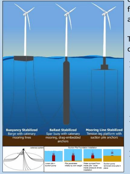
offshore wind energy. Newer designs aim to float turbines on the water surface to allow access to deeper waters.
